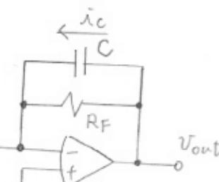
$$V_{out} = V_C, \quad i_C + \frac{V_{out}}{R_F} = -i_{in}, \quad i_C = C \frac{dV_C}{dt}$$
