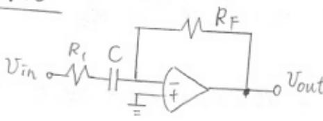
$$i_{in} = -i_f = -\frac{V_{out}}{R_f}$$
